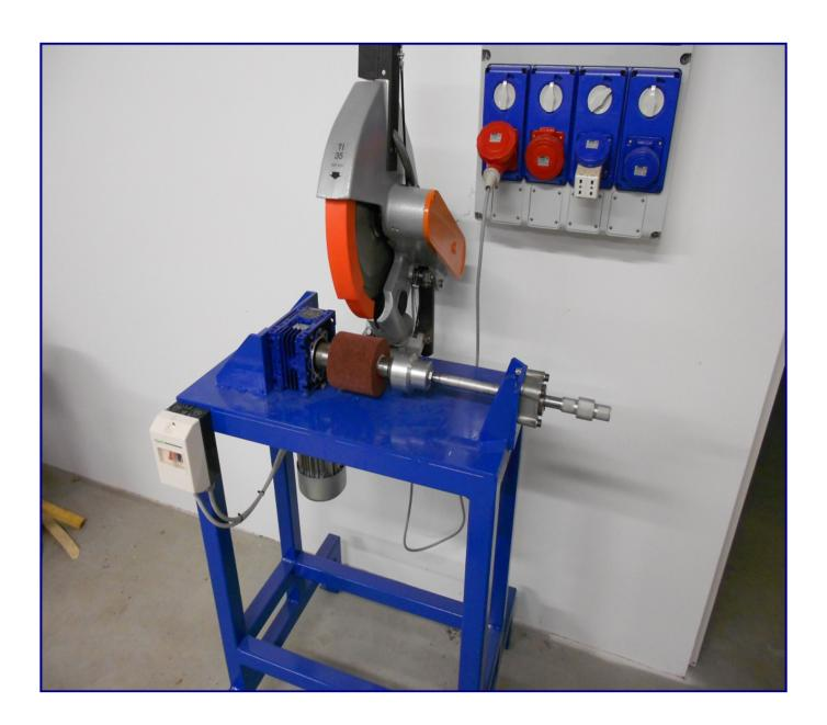
This is a manual cutting machine for 100x100mm wheels.
